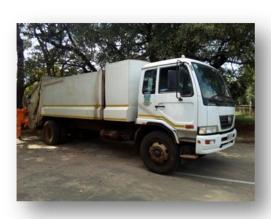
Figure 16: 11m3 Refuse Compactor Figure 17: 11m3 Refuse Compactor Truck stationed at Watervaal Region.
